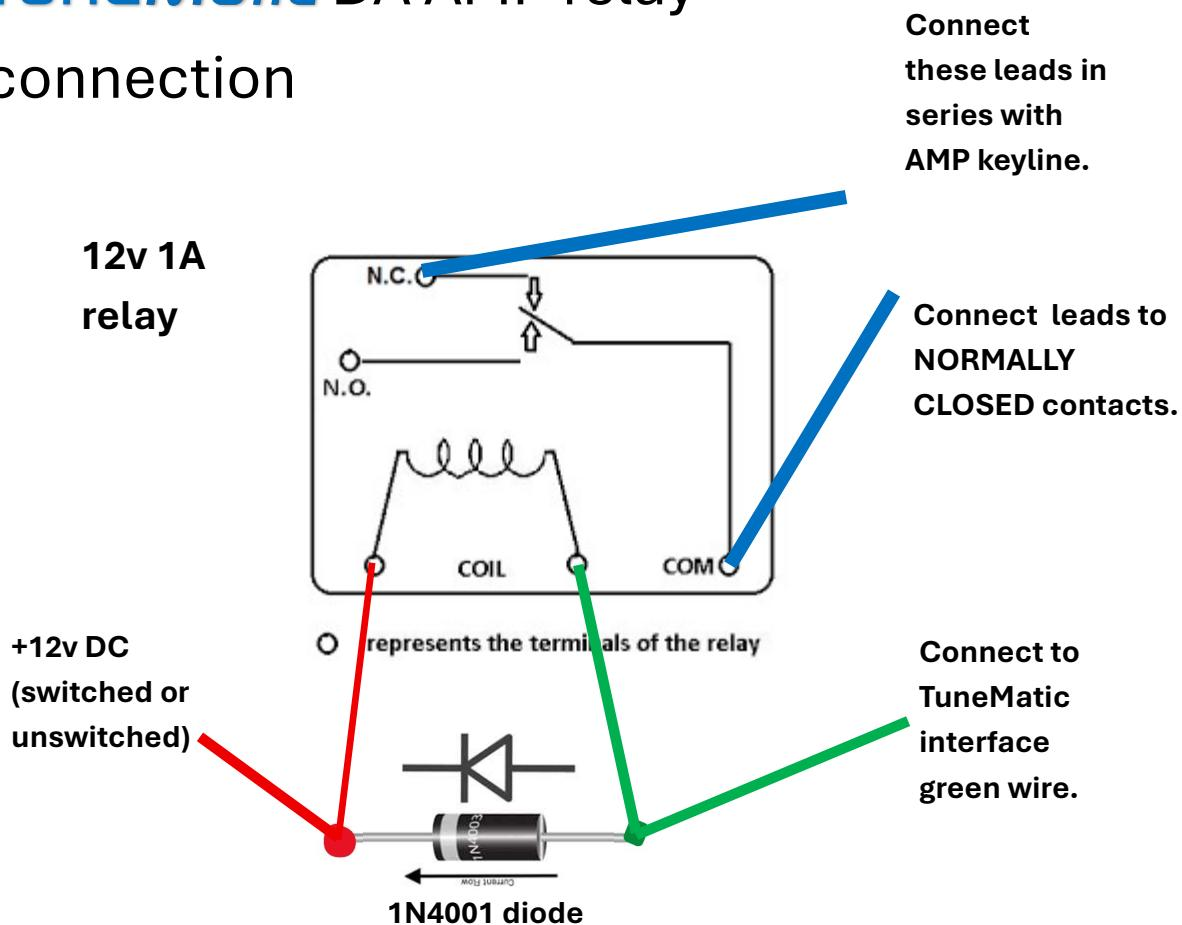
This circuit will allow the TuneMatic DA to unkey an external RF amplifier, allowing the amp to be bypassed when the TMDA is keying the transceiver.
